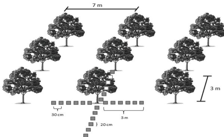
**Figure 3** Setup for the measurement of dry root biomass at each plot sized 20 x 20 x 20 cm and away from the tree base in 4 directions (North, South, East, and West), at 50 cm interval and up to 3 m in each direction.
